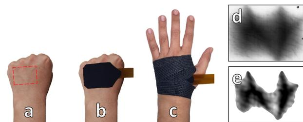
Fig. 1: a) Sensing area on the back of the hand showing the veins captured by the imager. b) Sensor system placed on the back of the hand. c) Sensor secured to the skin with a self-adhesive bandage. d) Original image retrieved by our sensor. e) Processed image highlighting the veins to facilitate hand posture and gesture recognition.
