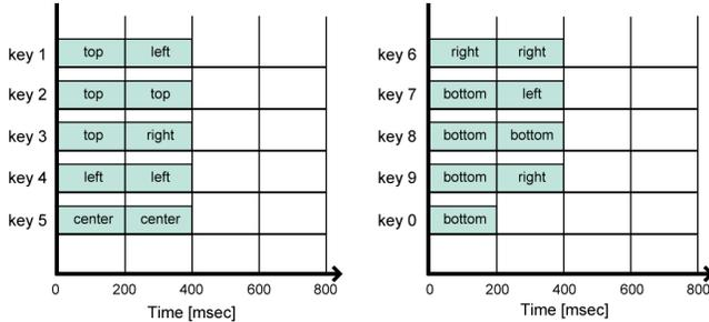
Figure 10: The mapping of the vibration patterns for the numeric keyboard used in the *Multiple Tactile* condition. Please note that the assignment of the vibration patterns is based on the spatial relationship of the keys (e.g., the combination of top and left vibration is assigned to key 1).
