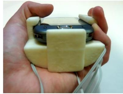
Figure 3: The special sleeve for the SemFeel prototype allowing placement of the vibration motors as close to the palm and fingers of users as possible.
