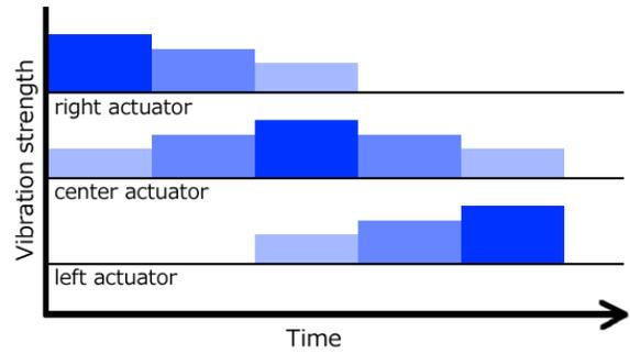
Figure 5: The smoothing of the vibration strength for the right-left vibration. The height of each square indicates the level of the vibration strength. The duration for each square is 200 [msec].
